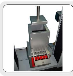
Industry standard test systems are available for a wide range of food products. Fixtures are available to perform compression, puncture, shear, extrusion and other tests. Calculated results for chewiness, toughness, ripeness etc. can be obtained directly from the tester or via a PC system.
