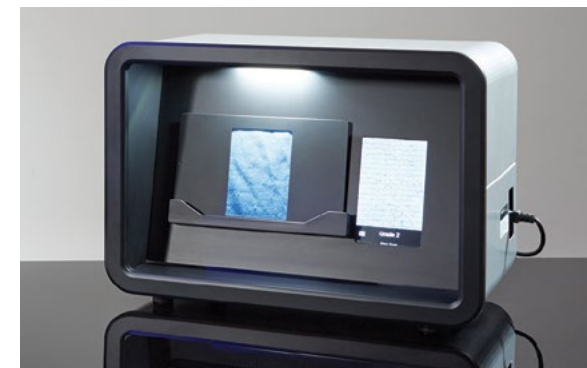
The library of images on the ProView include those to grade tests from the Martindale, SnagPod and ICI Pilling.
