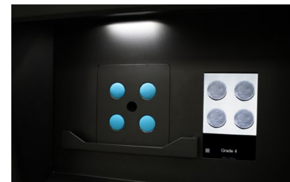
A range of sample holders and masks make the process of assessing and grading the samples clear.
