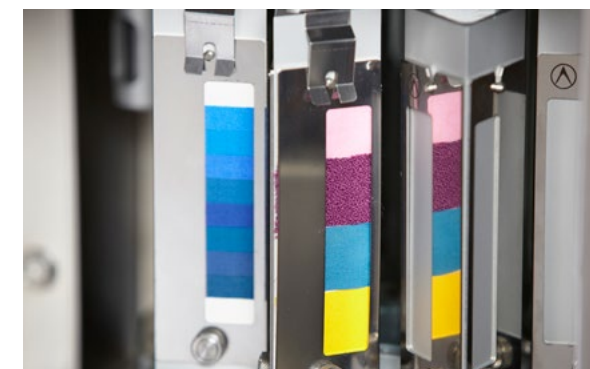
Our tri-sided sample holders are really easy to load and unload, and offer up to 1640cm 2 of useable exposure space.
