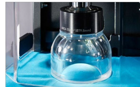
Accurate contactless laser distension measurement ensures pin point accuracy and extended diaphragm life.
