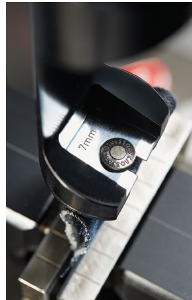
Stud Strength (T24) Suitable for testing buttons and tack-buttons (studs)
