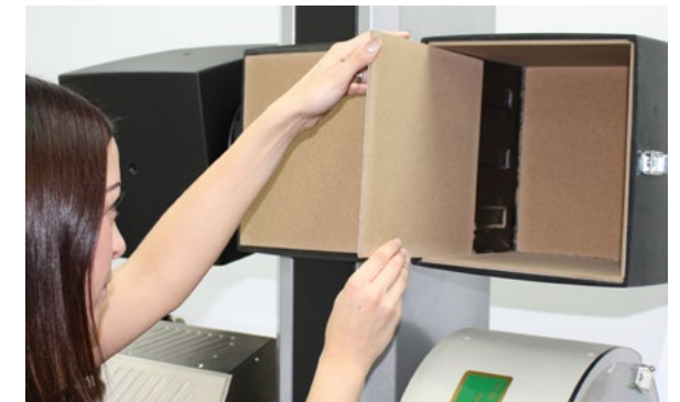
The magnetic qualities of the cork liners mean increased stability and tool-free fitting.
