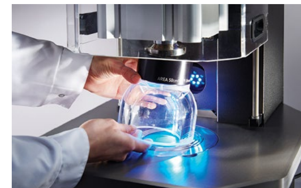
TruBurst has five interchangeable domes with automatic recognition of dome size, which accelerates testing and minimises downtime.
