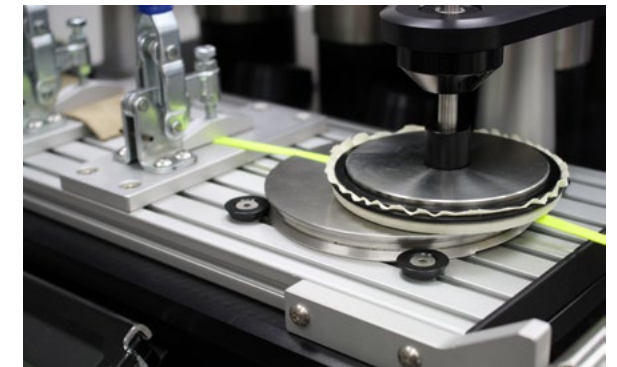
A table assembly is attached across both stations to test abrasive properties of multiples types of straps, ropes and shoelaces .
