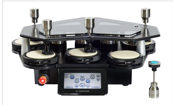
To accommodate mid-level use, the Midi-Martindale 1305 is equipped with 5 stations
