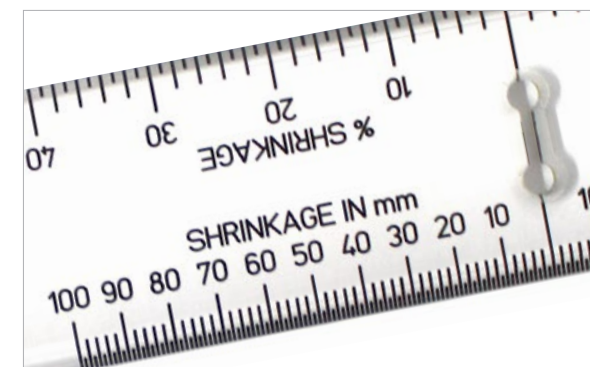
The James Heal stretch and recovery ruler measures percentage stretch and recovery without calculation.
