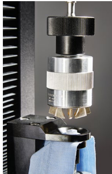
OctoGrip OctoGrip has 8 claws for gripping small attachments
