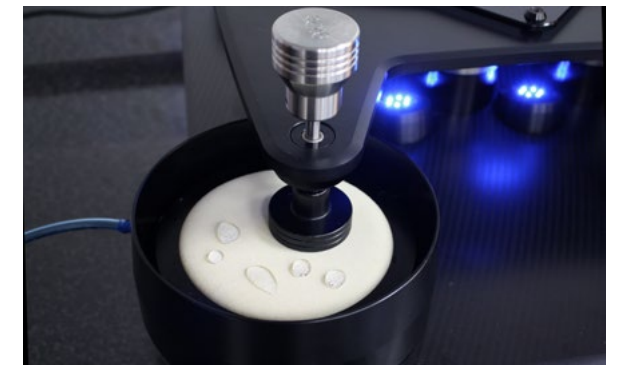
The water bath accessory is used to test products while damp or fully submerged in water.
