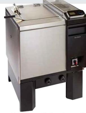
The new GyroWash<sup>2</sup> range comprises two machines: one with 8 and one with 20 positions. You can place either a small test vessel or a large test vessel in every position, so there is complete flexibility, should you wish to test to both ISO (small vessels) and AATCC (large vessels) standards.
