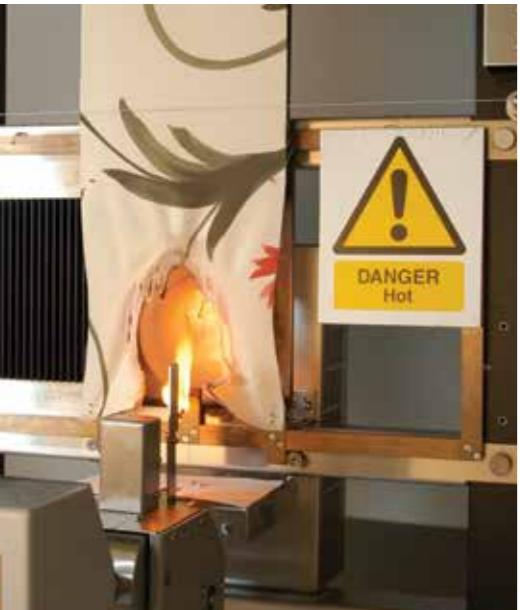
You can use FlexiBurn for testing the ignition and flame spread properties of apparel, curtains, drapes, nightwear, toys, protective clothing, technical fabrics, building and other materials.
