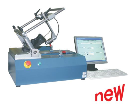
Longitudinal & torsional stiffness of complete footwear
