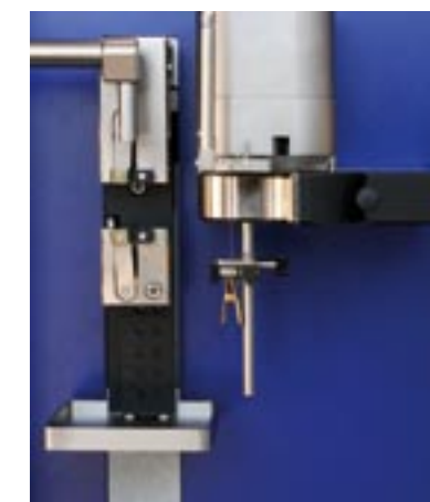
Fibre transfer from the vibroscopic measuring head to the tensile test section
