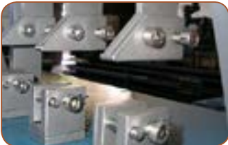
Sample holder fitted for standard ISO 5402
