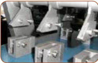
Sample holder fitted for standard ISO 32100
