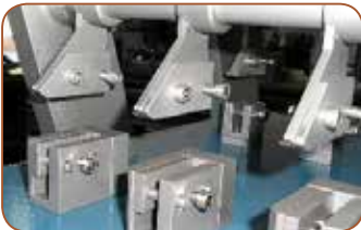
Sample holder for standard ISO 32100
