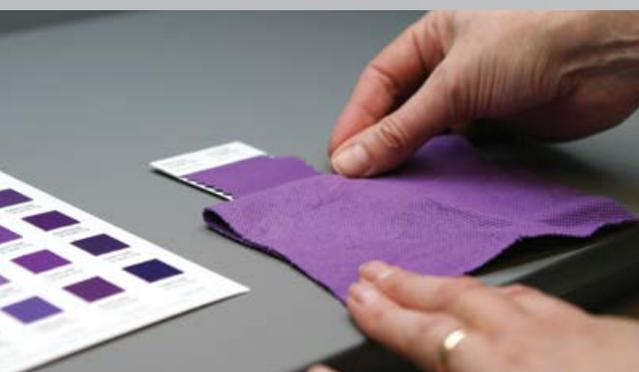
Colour requirements for manufacture and retail are complex and diverse. To ensure product colour, several types of light source are used (e.g. Artificial Daylight and a Point of Sale Light). Multiple light sources are also necessary to reveal colour inconsistencies and metamerism.
